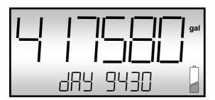
Full LCD display test feature illuminates all display segments and script text displays for 5 seconds when entering the program mode.
